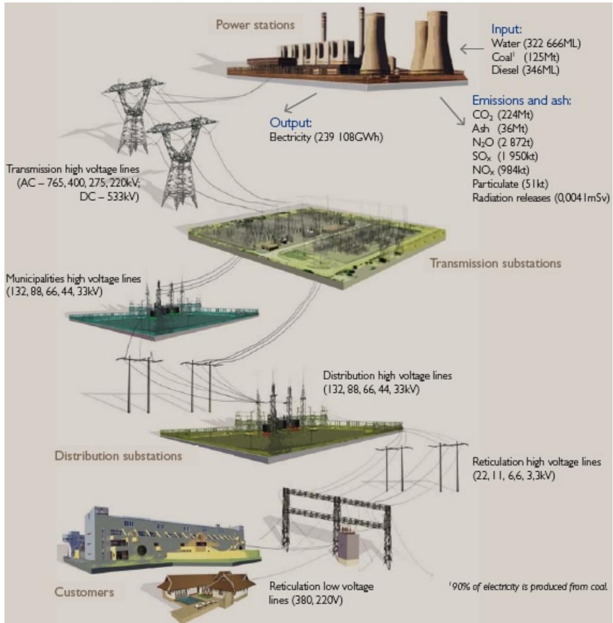
**Figure 3.1** Simplified electrical transmission and distribution system (source: [www.eskom.co.za](http://www.eskom.co.za))
