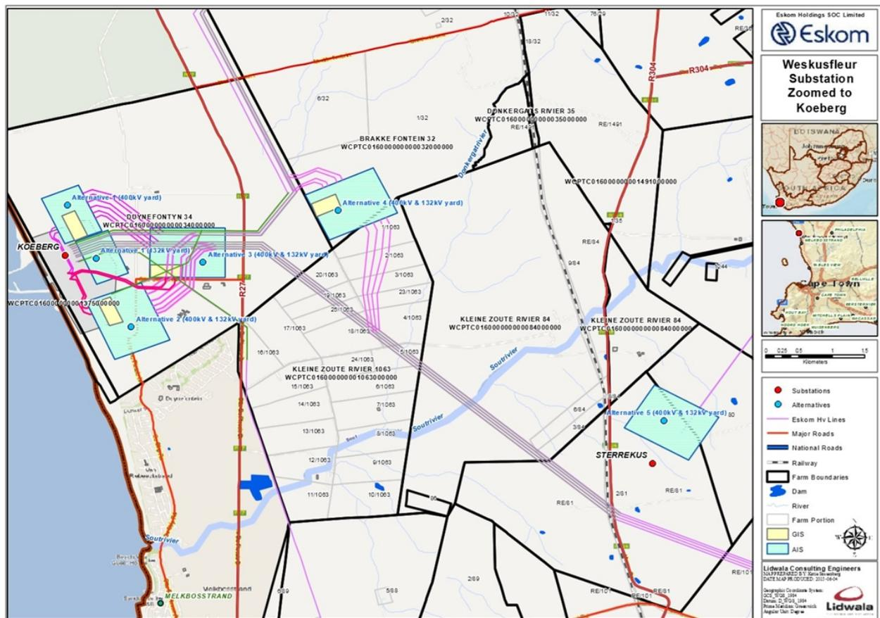
**Figure 3.7:** The 5 alternative sites within the study area (Note that the extent of the Air Insulated Substation (AIS) on the map is larger than required at 950 x 750 m, the actual required size is 760 x 550 m)
